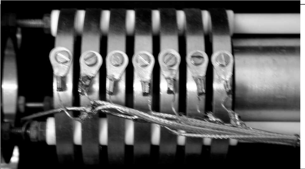
Figure 3.8: The MINERVA charge detectors are rather simple – They are just a series of plates
