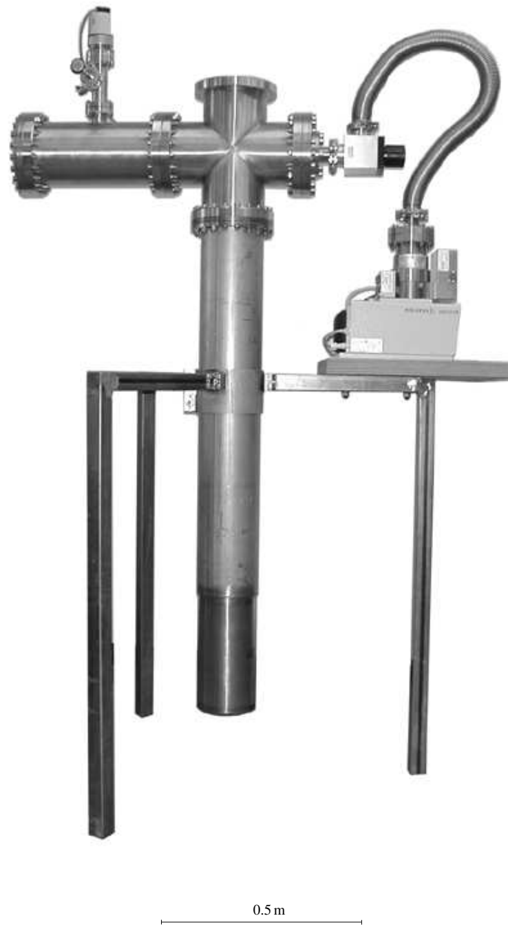
Figure 4.2: Photograph of the test setup with the vacuum pump and vacuum gauge. On the left hand side signal readout and power supply was connected.
