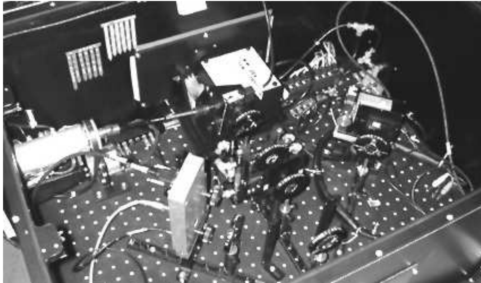
Figure 2.4: Setup for measuring the quantum efficiency of the photodiodes.
