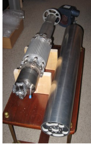
Figure 3.4: Picture of the neutron generator tube with its cooling fins on its outer sides (left) and the Al container (right).
