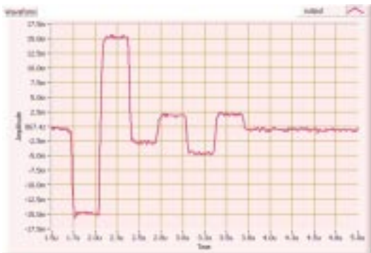
Figure 2.11: Readout chip output for one hit pixel. The six bins encode the address and the charge collected by the pixel (see text).
