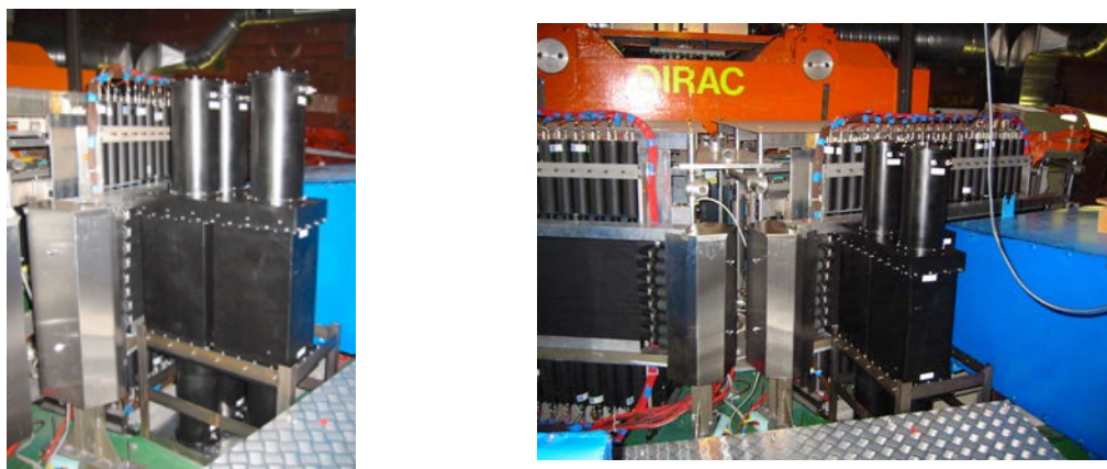
Figure 1.1: Photographs of the three aerogel modules (black) in the experimental area. The scintillation hodoscopes and the N_2 -Čerenkov counter (blue) are also visible.
